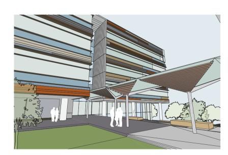
(MC1) Metal Cladding System Type 1: Cassette type metal cladding system. Finish and colour equal in appearance to Alpolic 'Medium Gray Metallic'.
