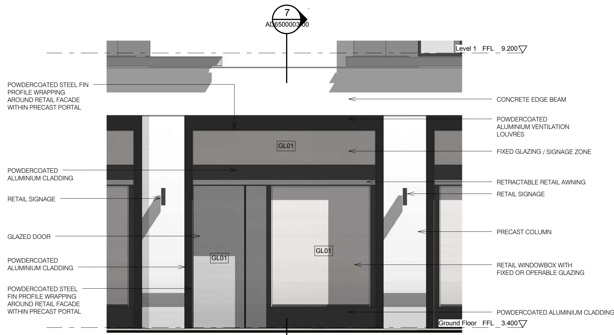
1 Typical Retail Facade Option A_Fixed Glazing 1 : 50
