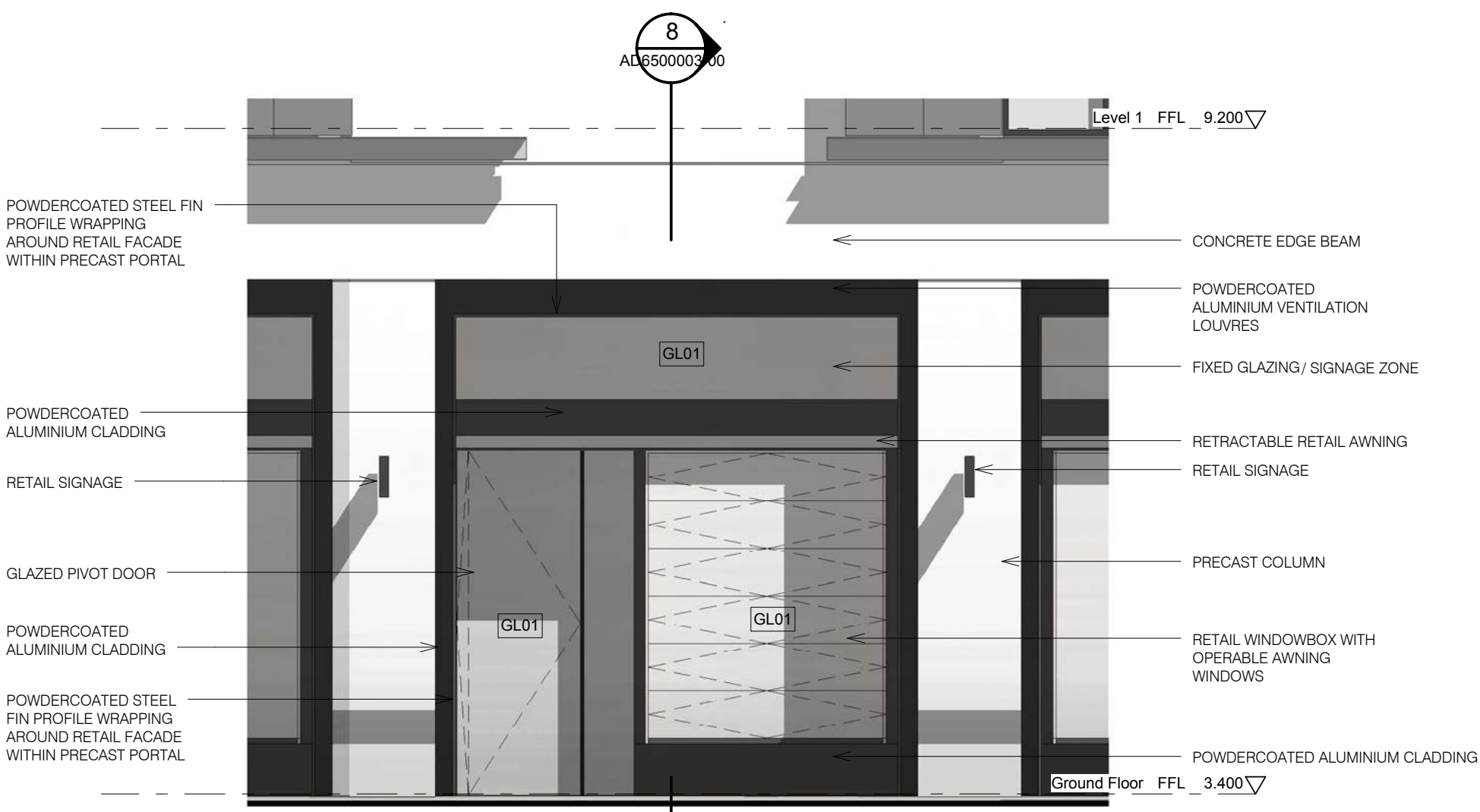
2 Typical Retail Facade Option B_Awning Windows 1 : 50
