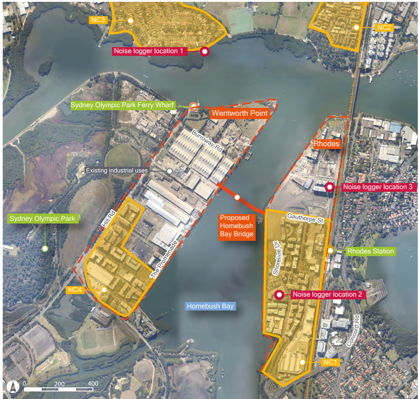
Figure 15.1 – Noise-monitoring locations and noise catchment areas
