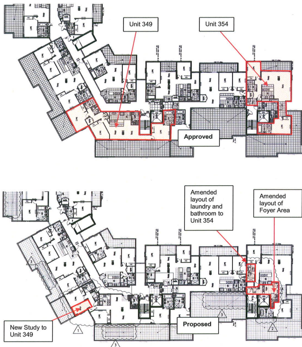
Figure 5: Approved and proposed layout of Units 349 and 354 and the Foyer in Building F
