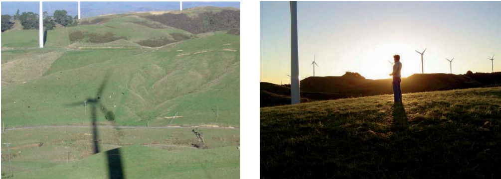
Example of shadow intensity variation with distance & turbine blocking small proportion of sunlight. (Source: Aurecon, 2011).
