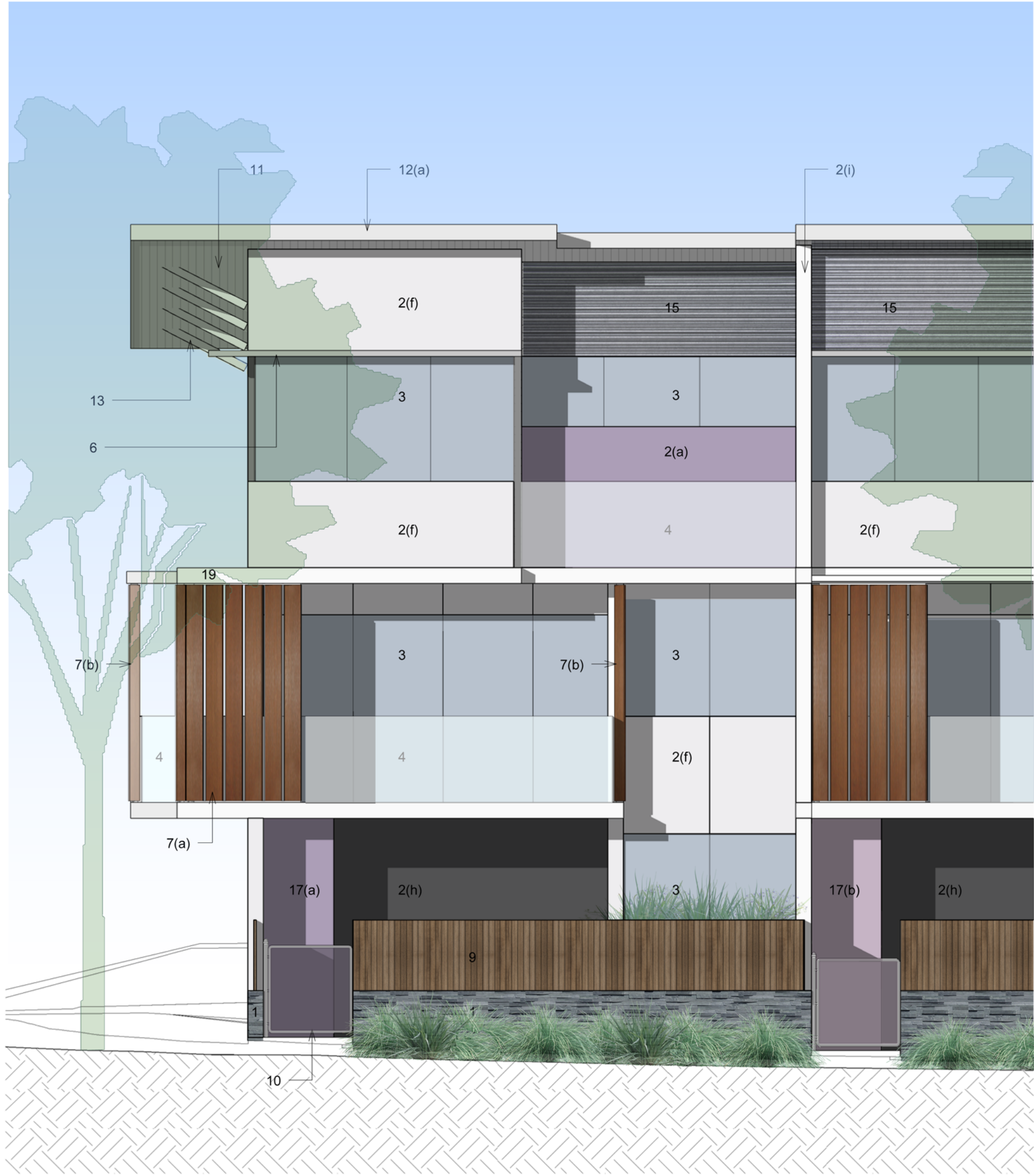
1 CALLOUT OF NORTH ELEVATION (BLDG 1) 1 : 50
