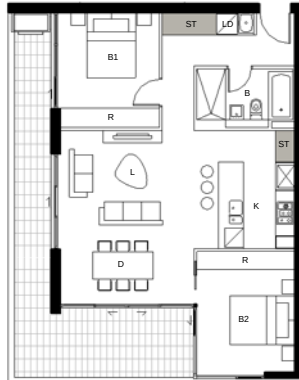
7 DETAIL PLAN BLDG A - Apartment Type 5 2 BED - 74sqm Storage - 4.8cbm
