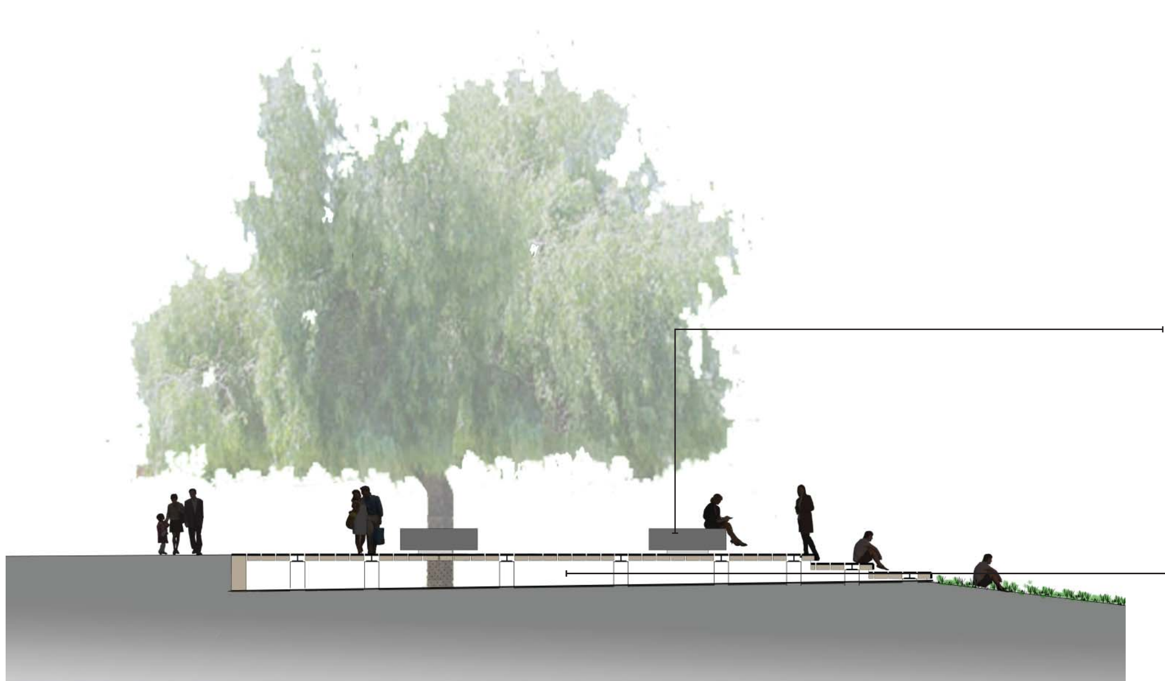
Suspended precast concrete unit deck with opportunities to integrate lighting and signage
