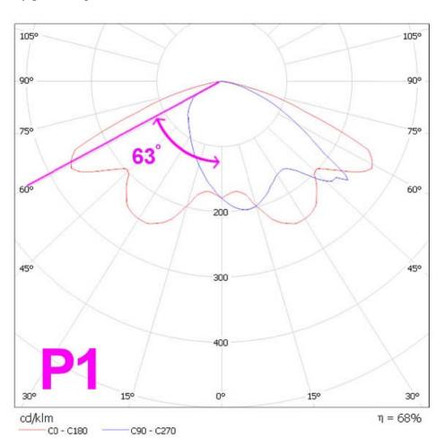
This shows that when using this luminaire no light is directed above 90°. Therefore at a viewing angle of 63° a value of 315 cd is shown.
