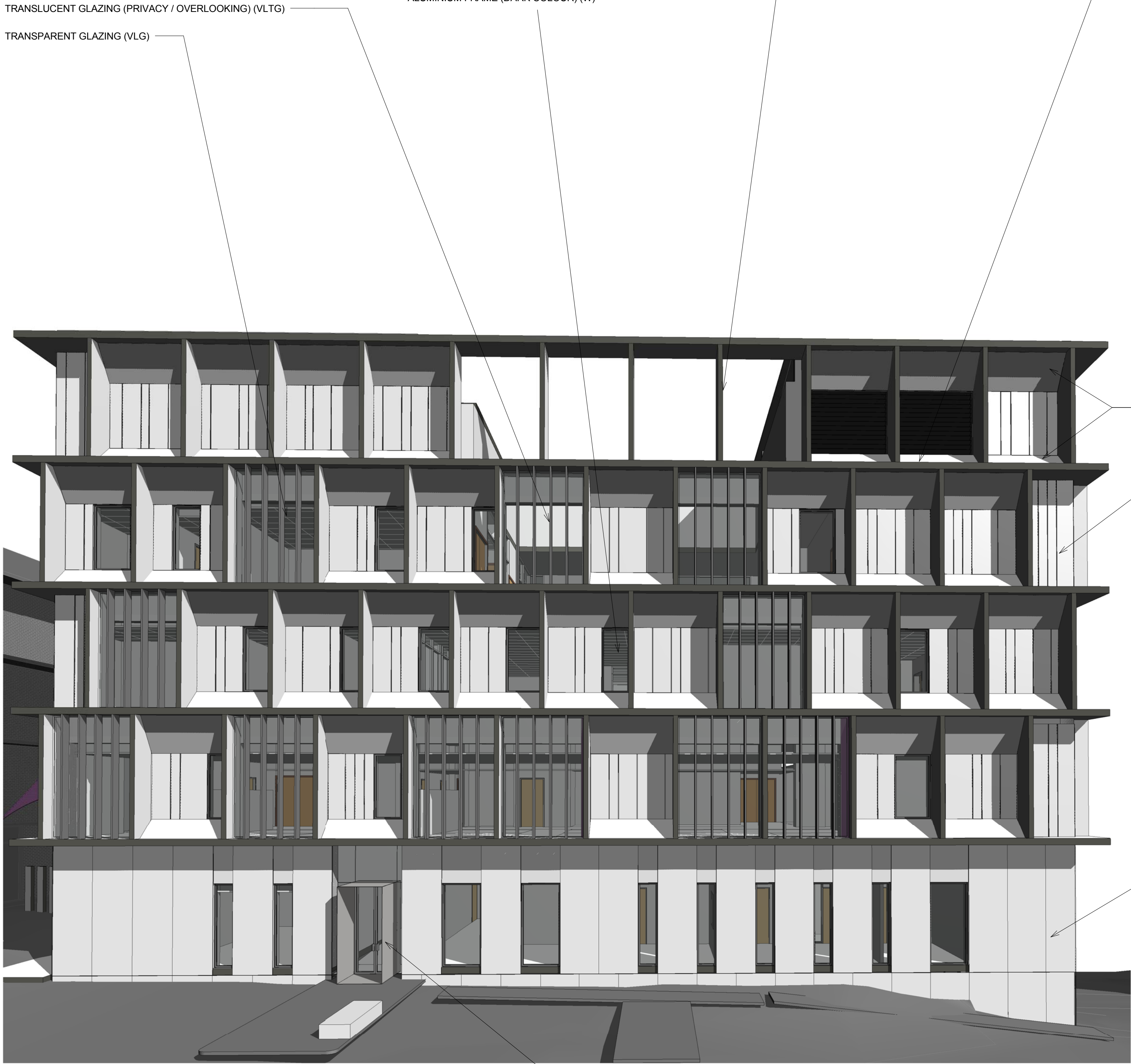
WINDOWS - TRANSPARENT GLAZED PANEL & POWDERCOATED ALUMINIUM FRAME (DARK COLOUR) (W)
