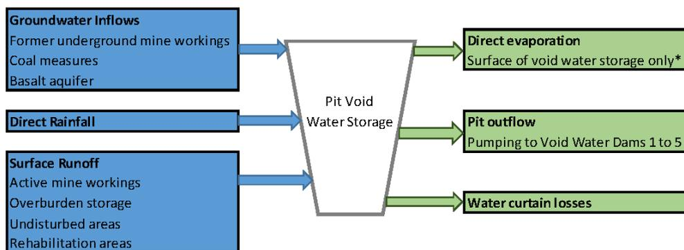
**Figure 1 Site Conceptual Water Balance**
