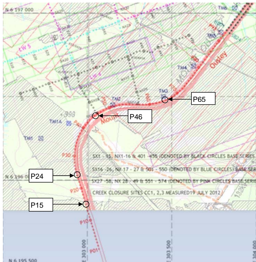
Figure 9 - Locations of Subsidence Related Cracking Observed on Mt Ousley Rd
