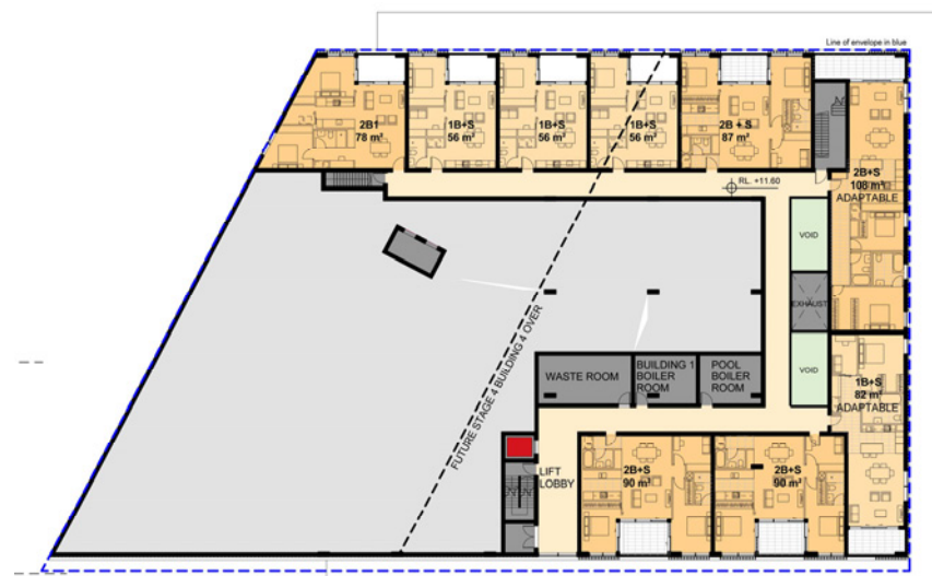
Figure 12 – First Floor Plan of Building 1B
