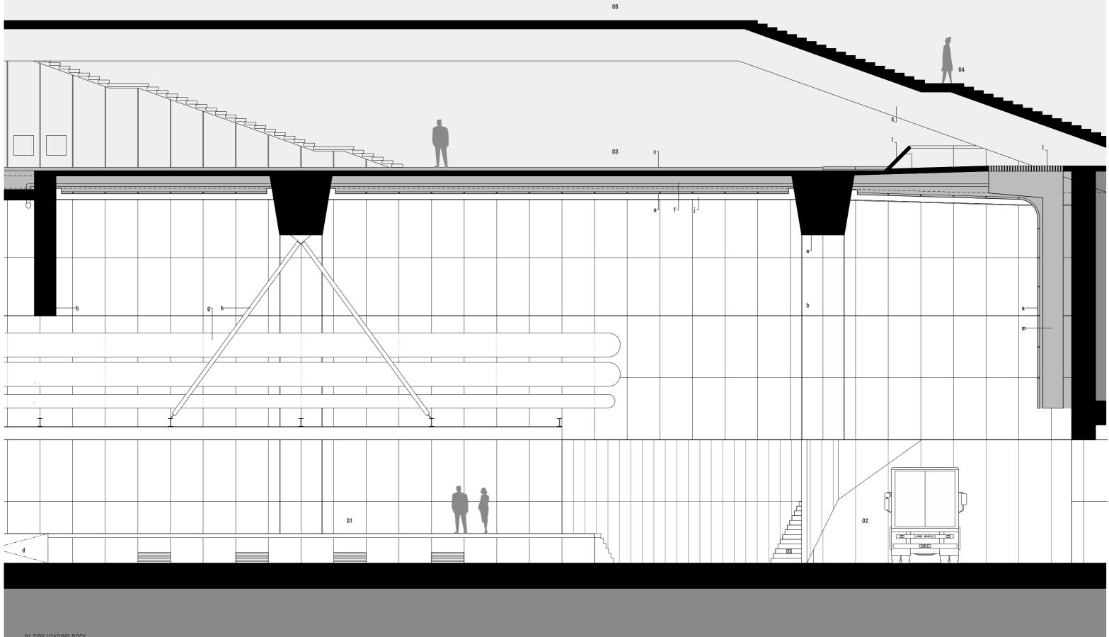
01 SIDE LOADING DOCK 02 TRUCK TURNING BAY BEYOND 03 VEHICLE CONCOURSE 04 MONUMENTAL STAIR 05 STAIR TO MECHANICAL PLANT ROOM 06 PODIUM a Compressed Fibre Cement Panels
