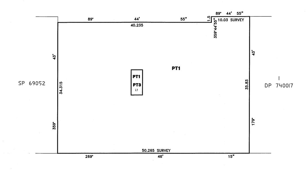
L1 PART LOT 3 IS LIMITED IN DEPTH TO A HORIZONTAL PLANE PASSING THROUGH THE CONCRETE FLOOR OF BASEMENT LEVEL TWO AND LIMITED IN HEIGHT TO A HORIZONTAL PLANE PASSING THROUGH THE CONCRETE FLOOR OF BASEMENT LEVEL ONE ABOVE PART LOT 1 EXISTS BELOW PART LOT 3 AND IS UNLIMITED IN DEPTH
