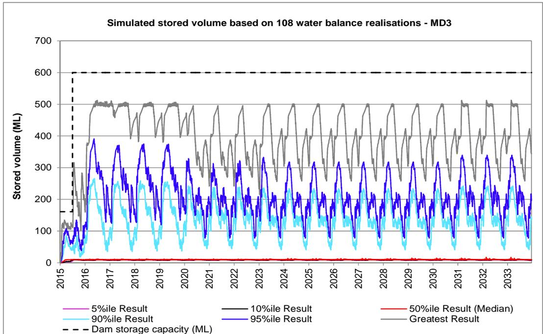
**Figure 4.5 Simulated time series of water stored in MW3**
