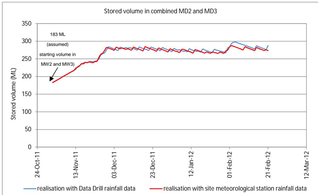
**Figure 4.9 Simulated volume of total water stored in MWDs (MW2 and MW3) from 1 November 2011 to 21 February 2012 – model verification**
