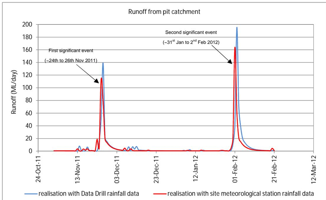
**Figure 4.7 Simulated contaminated runoff generated for pit catchment from 1 November 2011 to 21 February 2012 – model verification**
