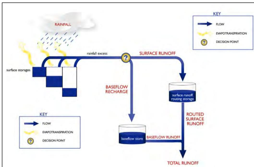
**Figure 2.4 Schematic layout of the AWBM rainfall-runoff model (Source: CRC for Catchment Hydrology, 2004)**
