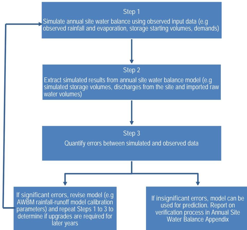
**Figure 6.1 Water balance model verification process**
