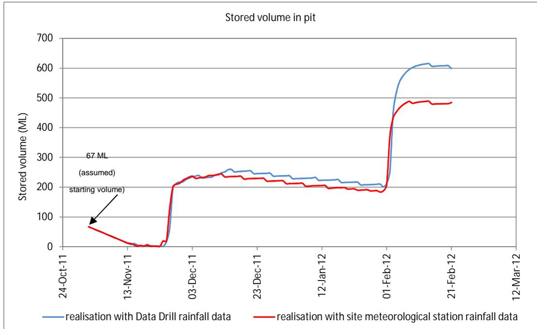
**Figure 4.8 Simulated volume of water stored in-pit from 1 November 2011 to 21 February 2012 – model verification**
