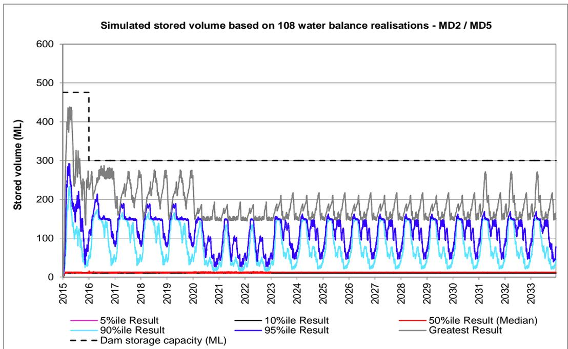
**Figure 4.4 Simulated time series of water stored in combined MW2 and MW5**
