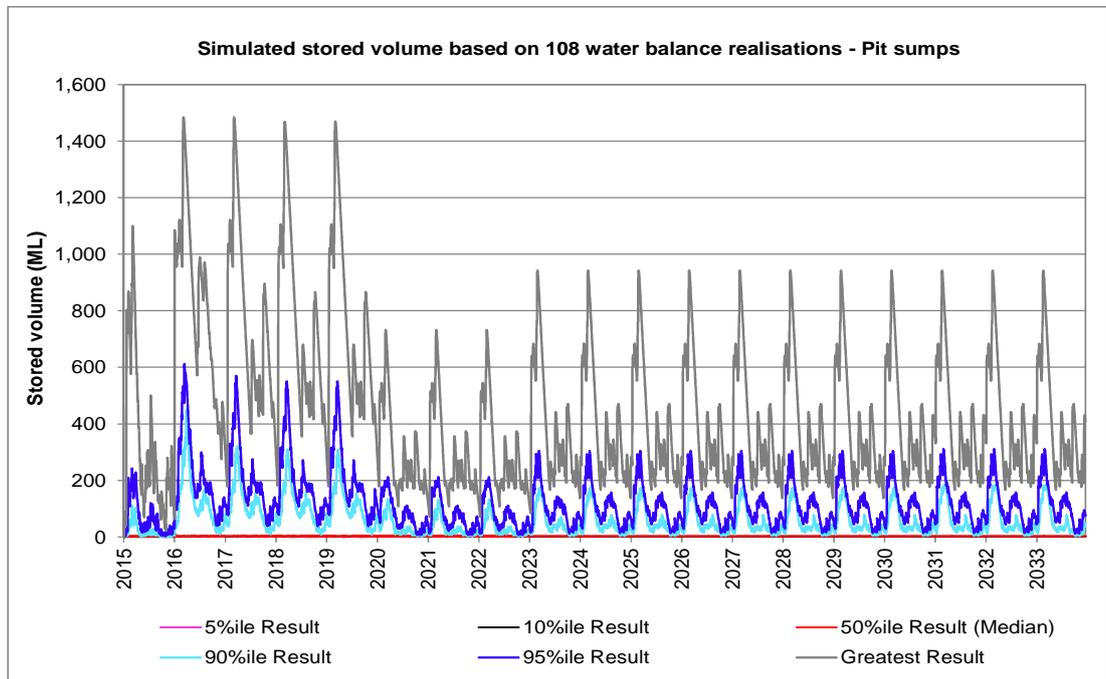
**Figure 4.2 Simulated time series of water stored in-pit sumps**
