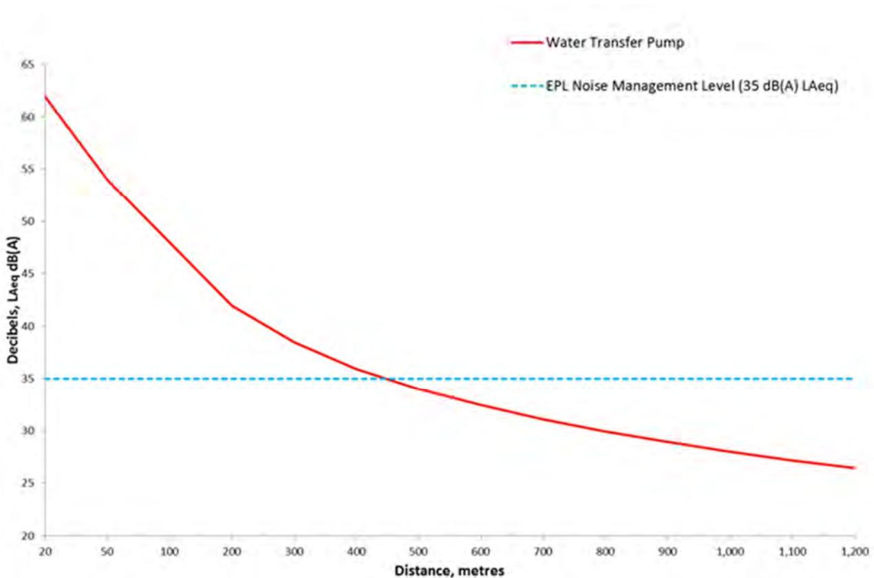
**Figure 6.8 Estimated noise levels at increasing separation distance from the pump**
