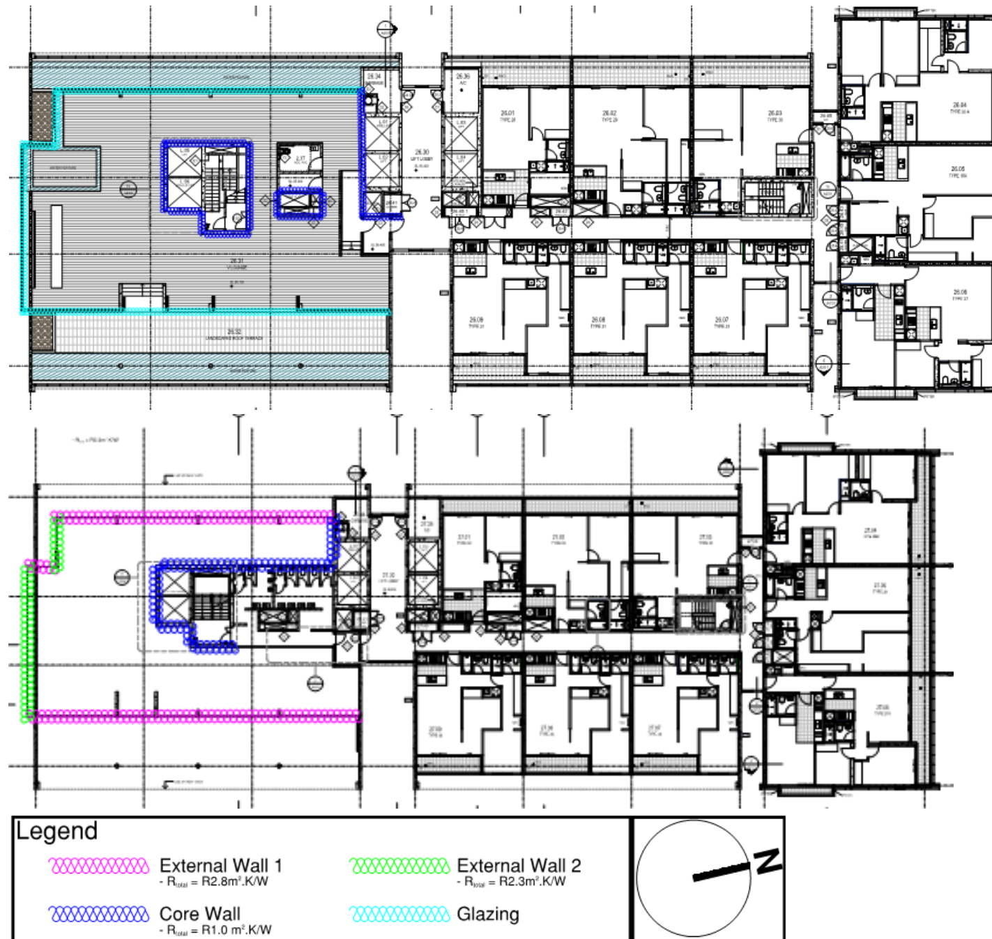
Figure 4: Level 26 [top] and Level 27 [bottom] wall insulation
