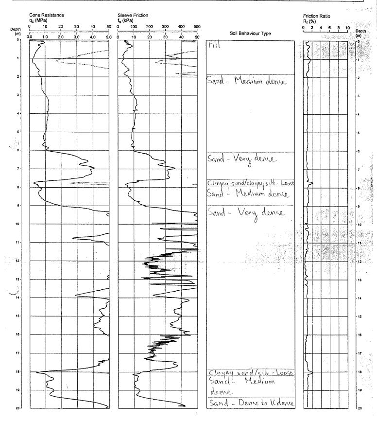
REMARKS: HOLE COLLAPSE AT 4.8 m AT COMPLETION OF TEST. \*LEVELLING TO BOREHOLE ON HOUSTON LANE TAKEN AS RL 25.9 m AHD.
