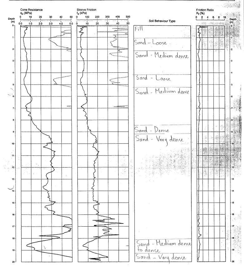
REMARKS: HOLE COLLAPSE AT 4.4 m AT COMPLETION OF TEST. \*LEVELLING TO BOREHOLE ON HOUSTON LANE TAKEN AS RL 25.9 m AHD.
