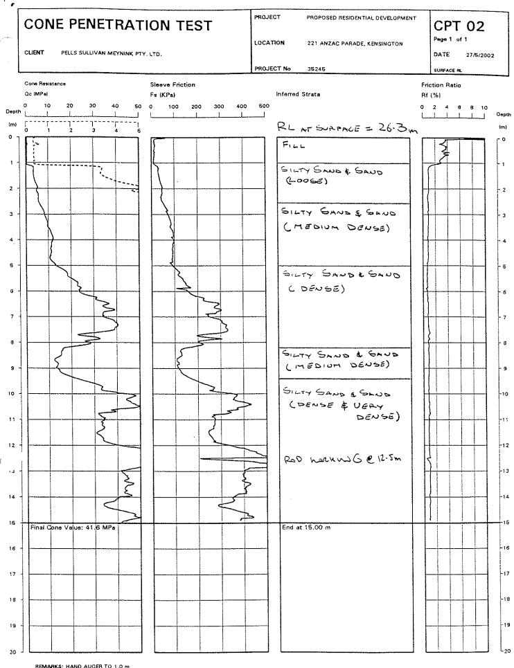
REMARKS: HAND AUGER TO 1.0 m HOLE COLLAPSE AT END OF TEST: 1.1 m
