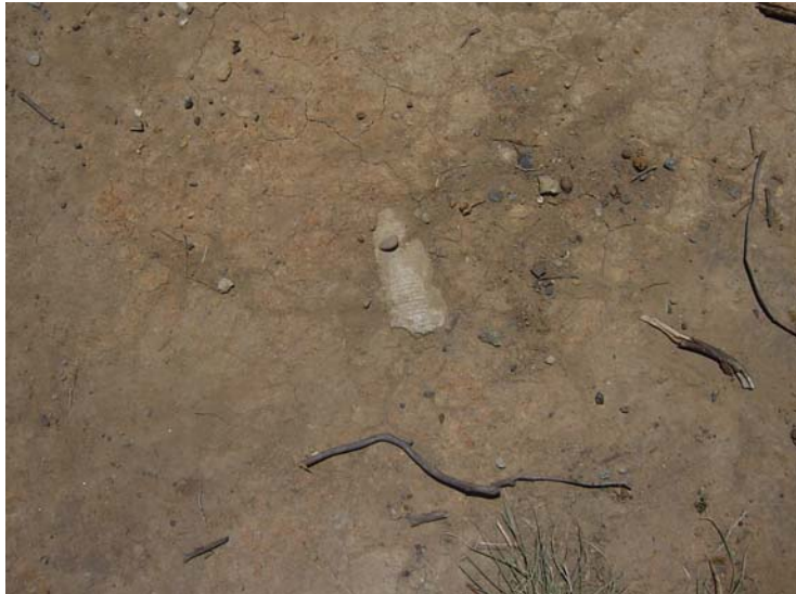
Possible fragment of cement bound asbestos in exposed soil to the south of East Block
