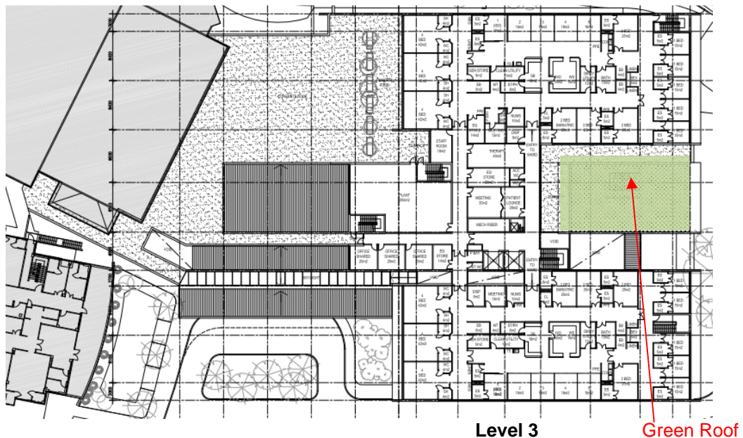
Green Roof over Metal sheet roofing
