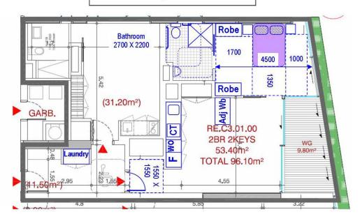
AS4299 Clauses 4.3.1, 4.3.2 and 4.3.3 **Accessible entry** – The front entrance to these units provides at least 1550mm X 1550mm externally in the common corridors and internally with 520mm minimum latch side clearance, which complies with the spatial requirements of AS4299.
