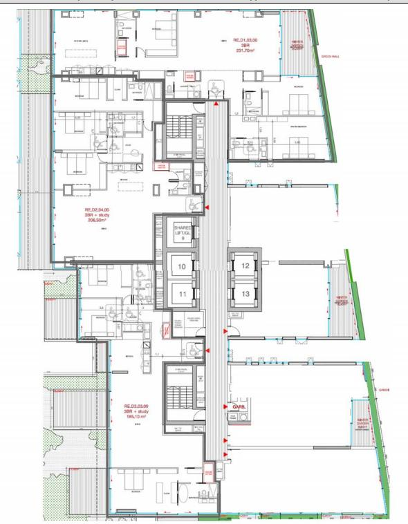
AS4299 Clauses 4.3.1, 4.3.2 and 4.3.3 **Accessible entry** – The front entrance to this unit provides at least 1550mm X 1550mm externally in the common corridor and internally with 520mm minimum latch side clearance, which complies with the spatial requirements of AS4299.
