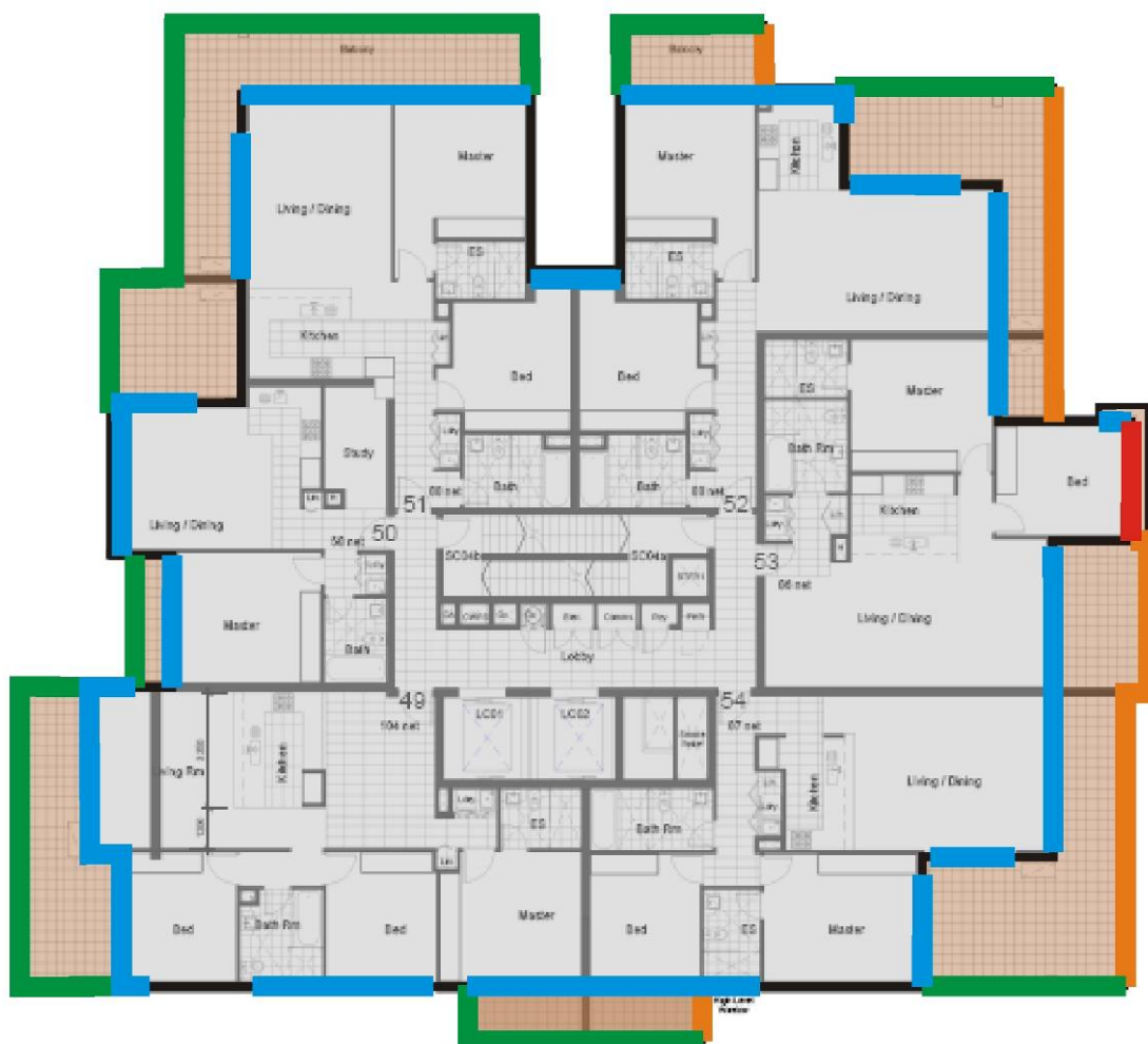
Figure 3: Recommended Reflectivity Properties of the Glazing for a Typical Level of the Residential Tower
