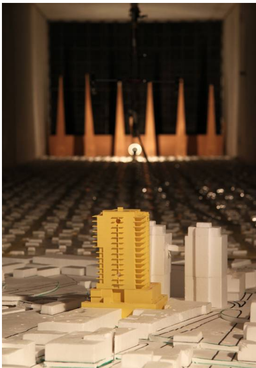
Figure 1c: Photographs of the Wind Tunnel Model (model with the development, views from the south and east)
