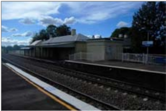
Buildings of the up platform at Greta Railway Station. Note the addition of a concrete riser on the easterly end of the platform to facilitate boarding modern passenger cars.
