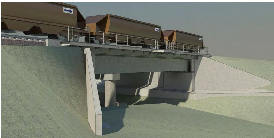
Figure 7.38 Proposed Jump Up Creek Underbridge 3D Schematic
