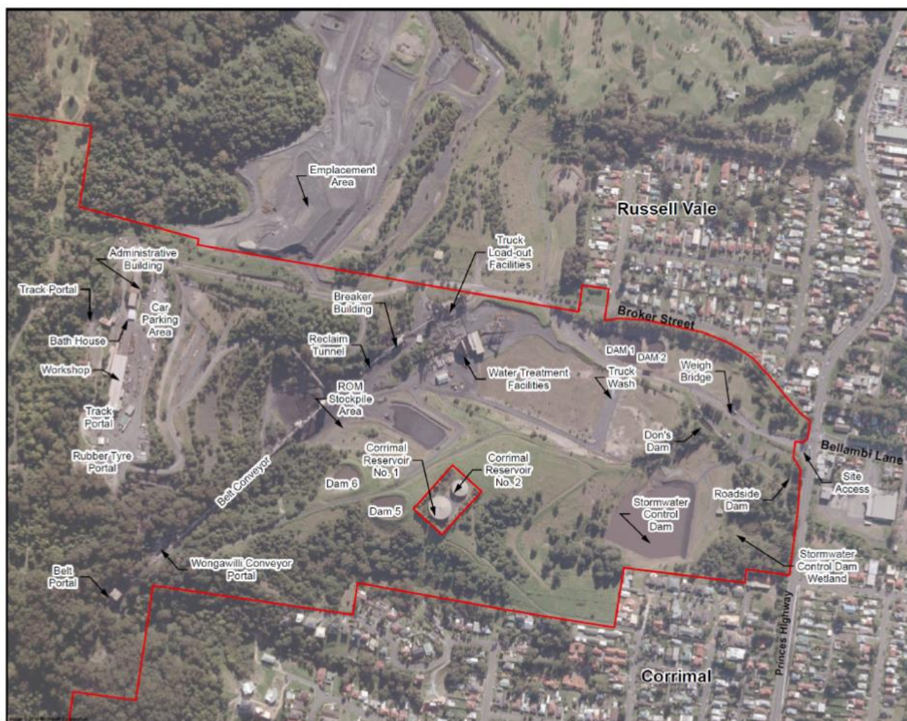
Figure 4: Pit top surface facilities
