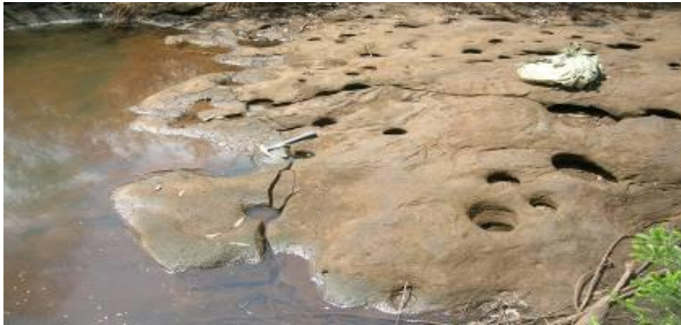
Photograph 20.4 Bed cracking adjacent to a pool in Wallandoola Creek (WC4) (GeoTerra, 2012a)
