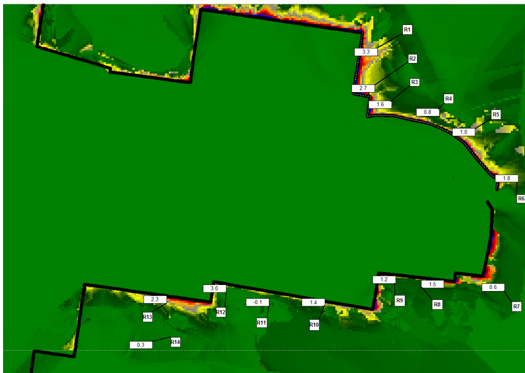
Figure 7-2: Barrier Attenuation at 1.5m Above Ground - Full Perimeter 4m Barrier, Neutral Meteorological Conditions, Year 4, Day & Evening
