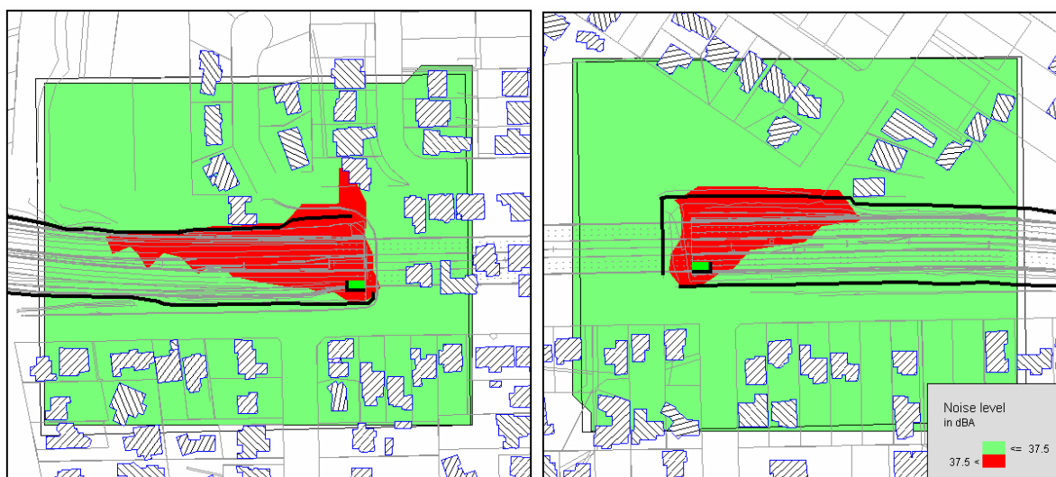
Figure 13 Activity C – Widening within Westbound Tunnel (Night-time 37.5 dBA NML) – Shed and Curtain in Place
