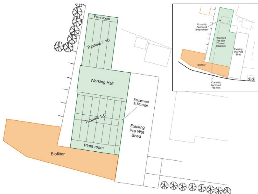
Figure 3: Proposed Pre-wet Tunnel Structure and Biofilter (inset approved biofilter and pre-wet shed overlaid with proposed modification)
