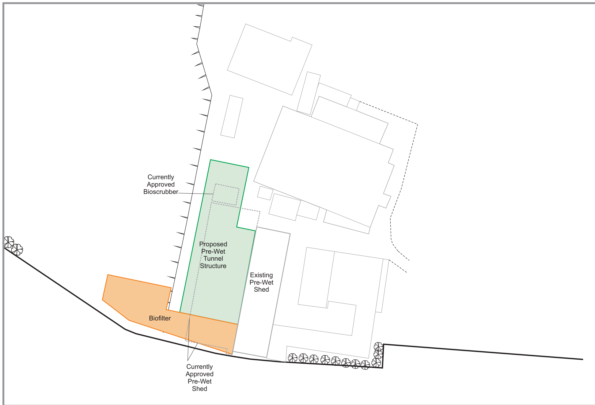
FIGURE 3 Proposed Pre-Wet Structure and Biofilter
