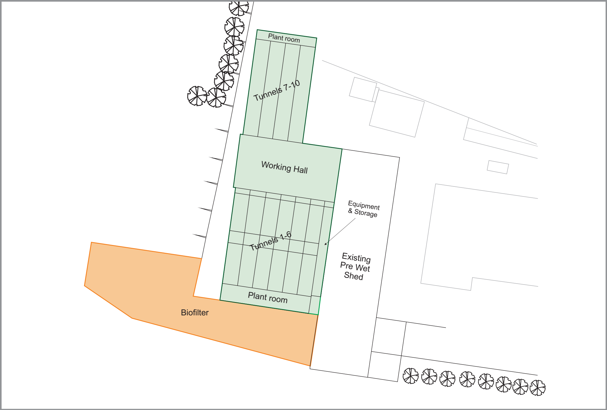
FIGURE 4 Internal Layout of Proposed Pre-Wet Structure
