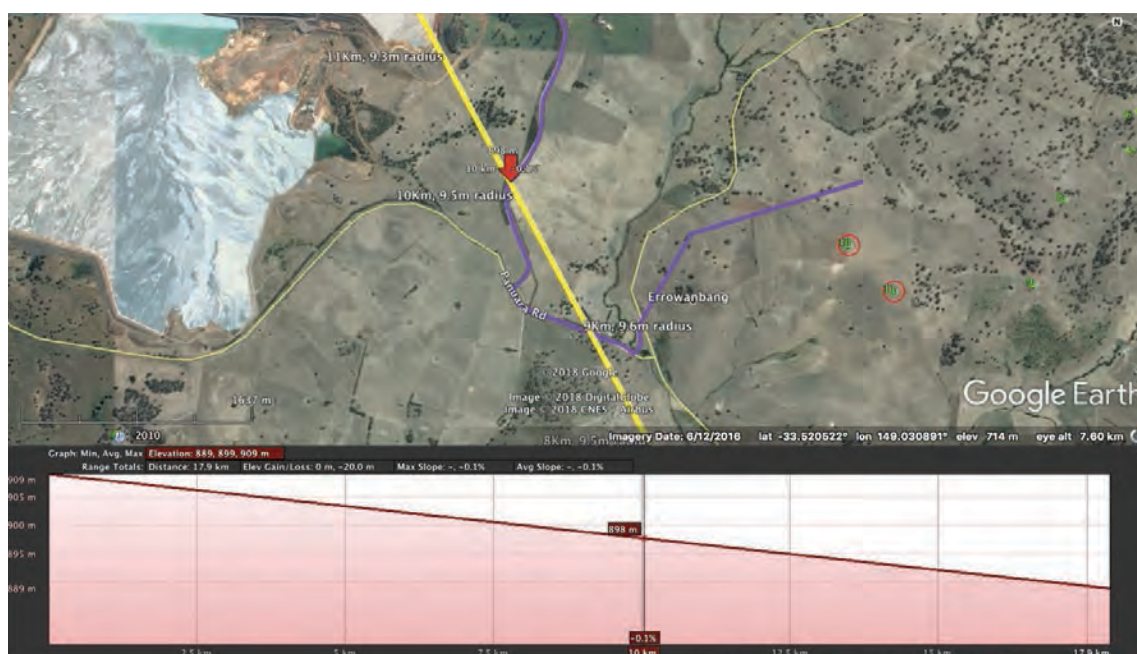
Figure 4-38 Path E - Ray line at the transmission line crossing is at 898 m
