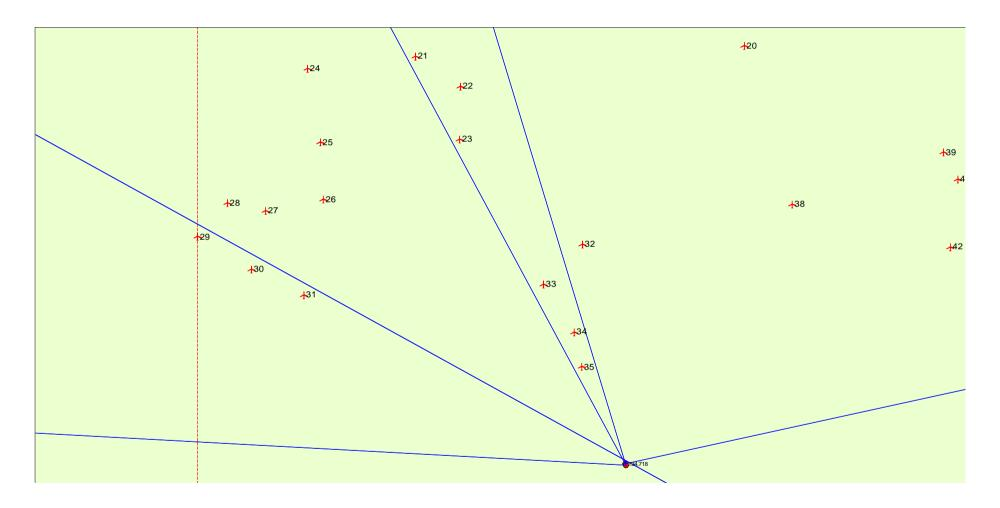
204434 9001068 Frequency (MHz) = 15000.0 K = 1.33 Fn = 1.00, 2.00 Latitude 33 27 20.17 S Longitude 148 59 09.60 E Azimuth 151.76° Elevation 883 m ASL Antenna CL 10.0 m AGL 33 35 50.34 S 149 04 37.11 E Longitude Azimuth 331.71° 885 m ASL Elevation Antenna CL 25.0 m AGL Lawrence Derrick & Associates Optus Link Nov 22 10
