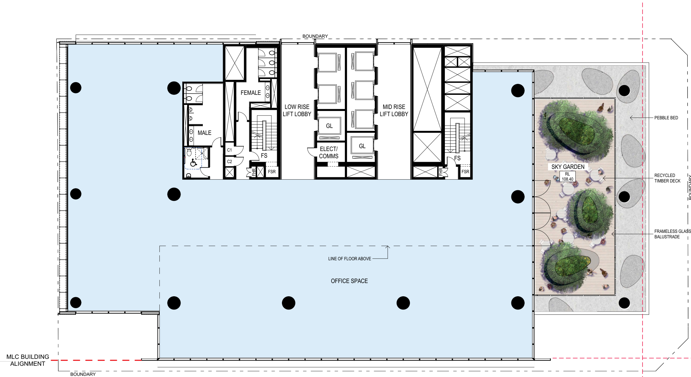
Approved: Level 20 - Low Rise Transfer Level FFL: 108.20 GFA: 1036 m 2 GBA: 1198 m 2
