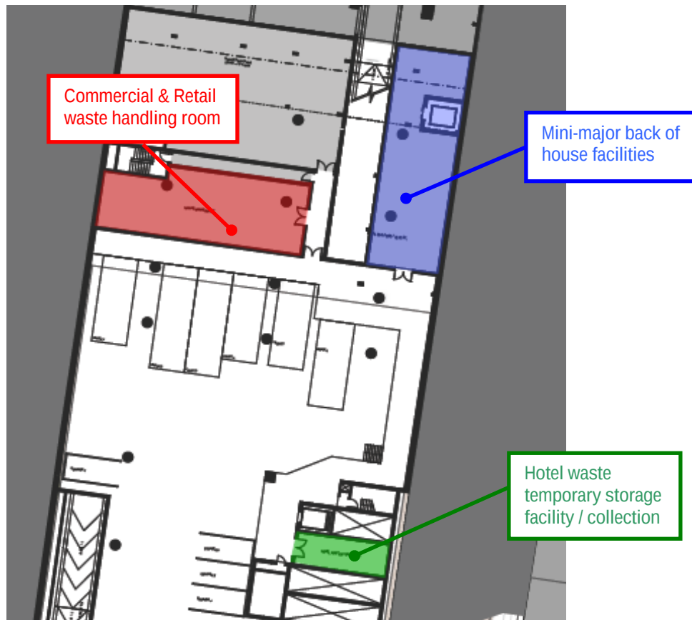
Figure 5: Lower Ground Waste Handling Facilities
