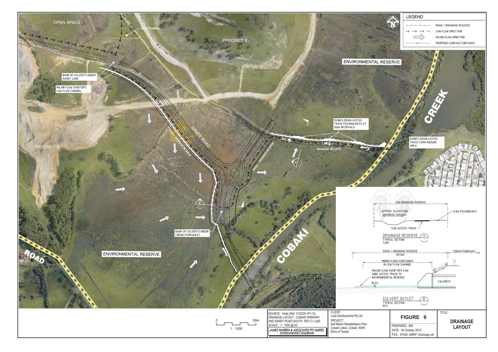
The proposed Saltmarsh rehabilitation works include measures to promote tidal exchange through re-engineering existing levee and drainage systems and some regrading works. More details are provided in **SECTION 6.2.2**. By controlling, repairing and improving the surface water management within the rehabilitated areas, the mosquito and biting midge problem is controlled.
