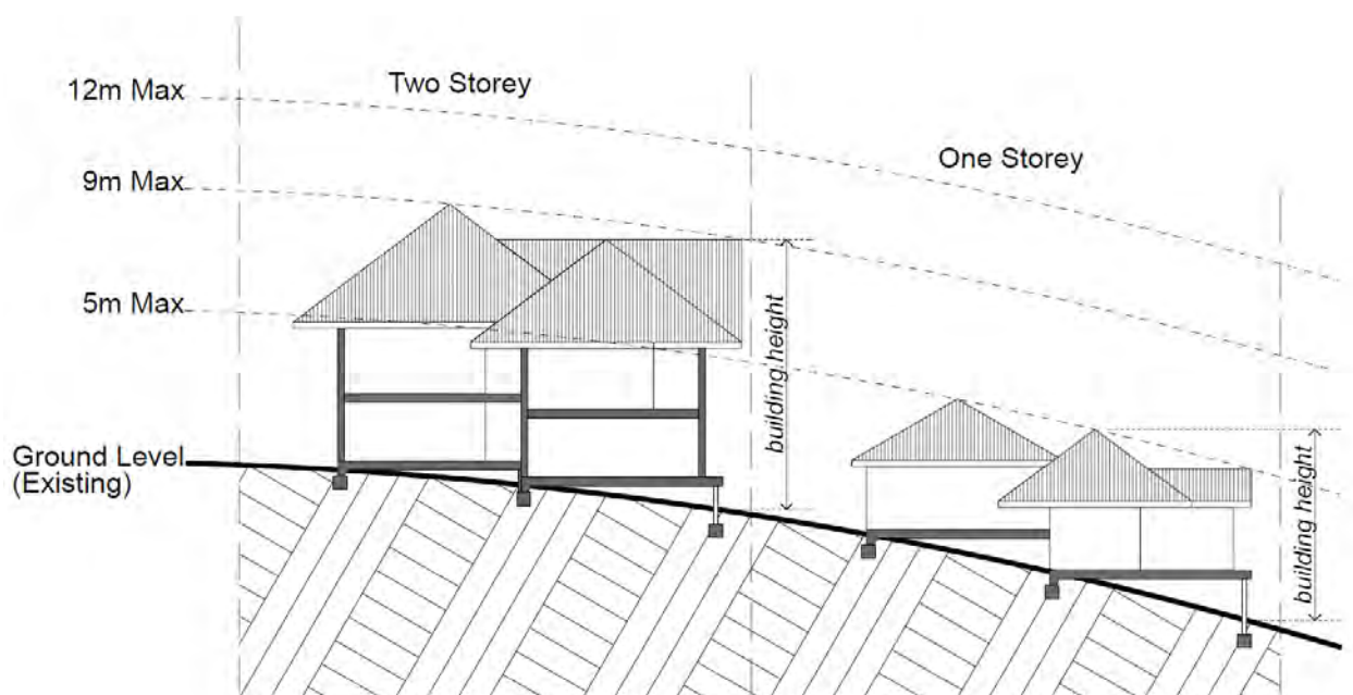
Figure 2.2.4.1 Overall Building Height
