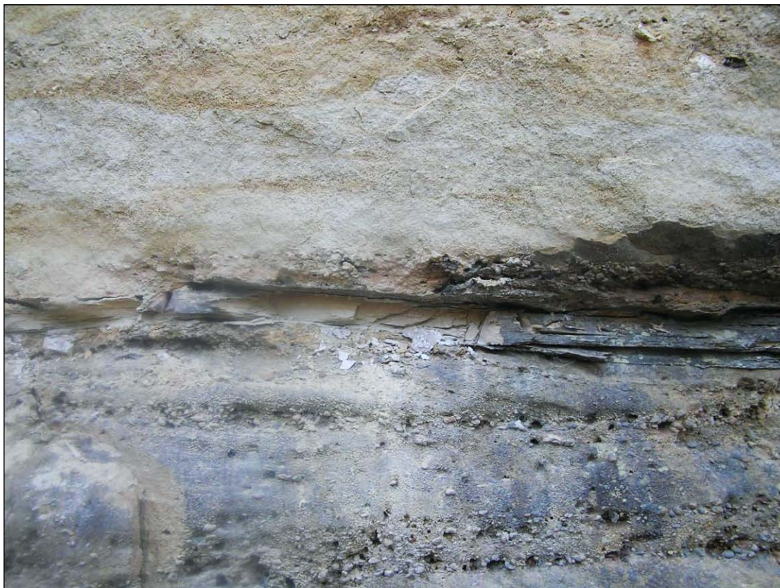
Figure 8: Examples of perceptible shear movements.
