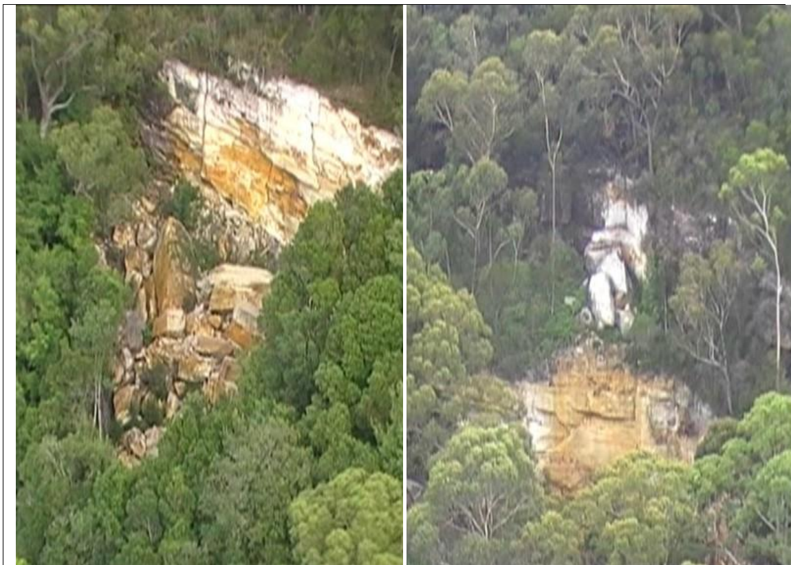
Figure 39: Falls of Ground over Dendrobium Colliery that the Panel Considers Constitute Cliff Falls.
