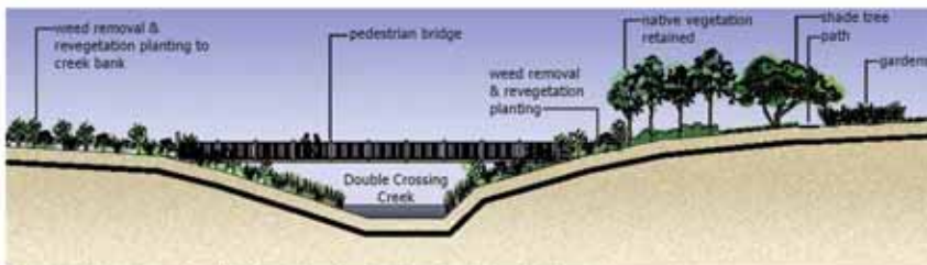
E Typical Section - Double Crossing Creek & pedestrian bridge
