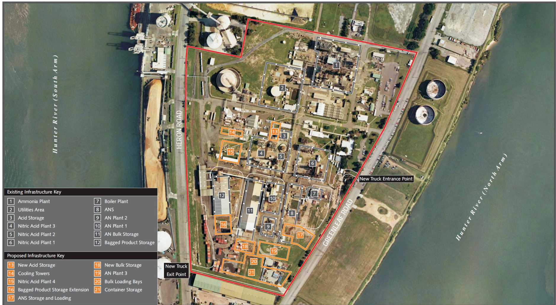
Figure 1.2 Proposed Site Layout Orca Australia Pty Ltd Environmental Assessment Proposed Ammonium Nitrate Facility Expansion Greenleaf Road, Kooragang Island
