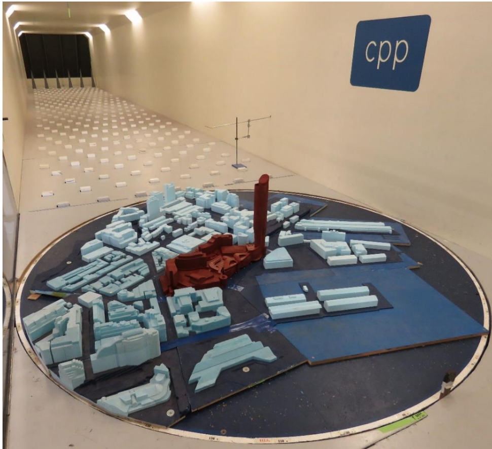
Figure 7: The Star model in the wind tunnel viewed from the south-east, proposed configuration
