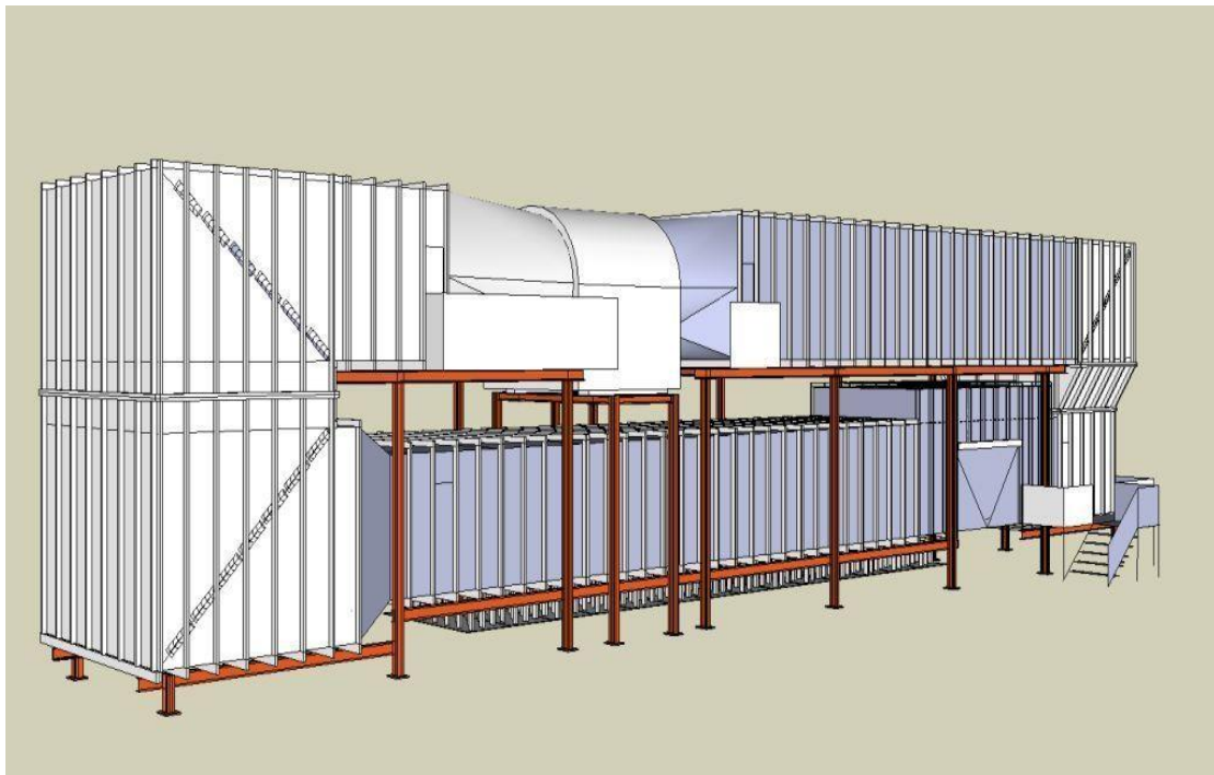
Figure 2: Schematic of the closed-circuit wind tunnel
