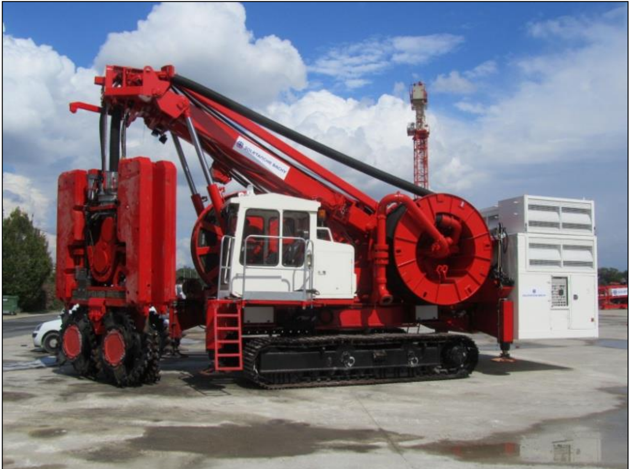
Plate 5: Mini-hydrofraise (Photograph courtesy of Menard Oceania)
