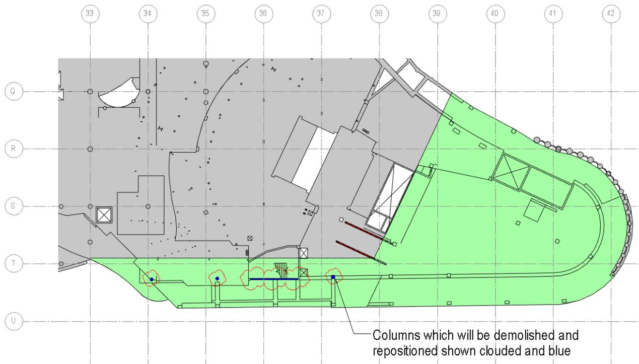
Figure 3 - Proposed Demolition Extent at Level 0 (demolition shown green)
