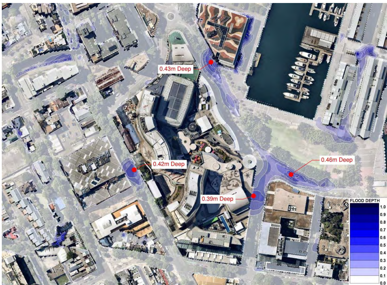
Figure 9. Existing 100 Year ARI Flood Depths With Amended Pit Blockage Factors
