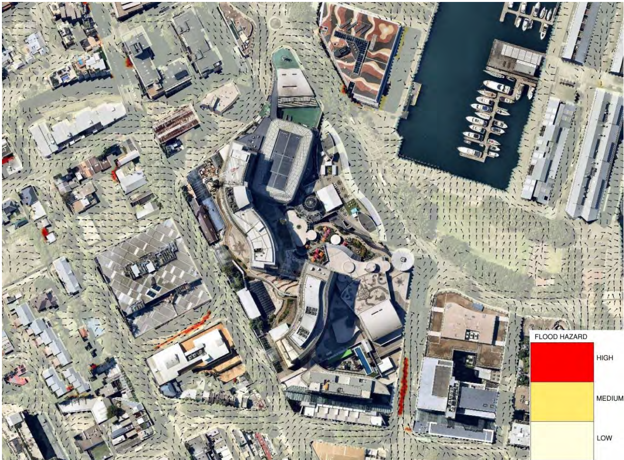
Figure 10. Existing 100 Year ARI Flood Hazard With Amended Pit Blockage Factors
