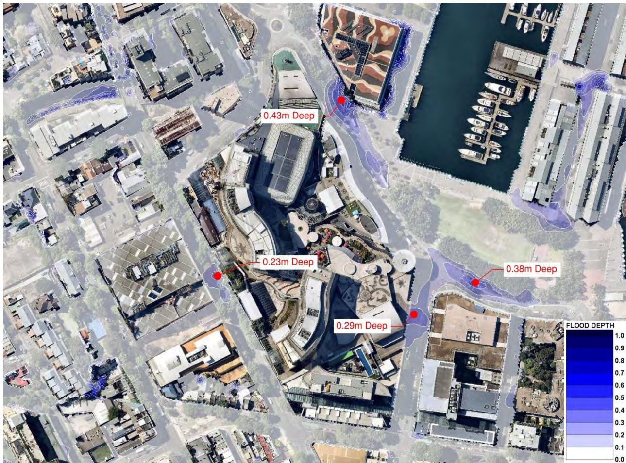
Figure 15. Proposed 100 Year ARI Flood Model Results With Stormwater Upgrades
