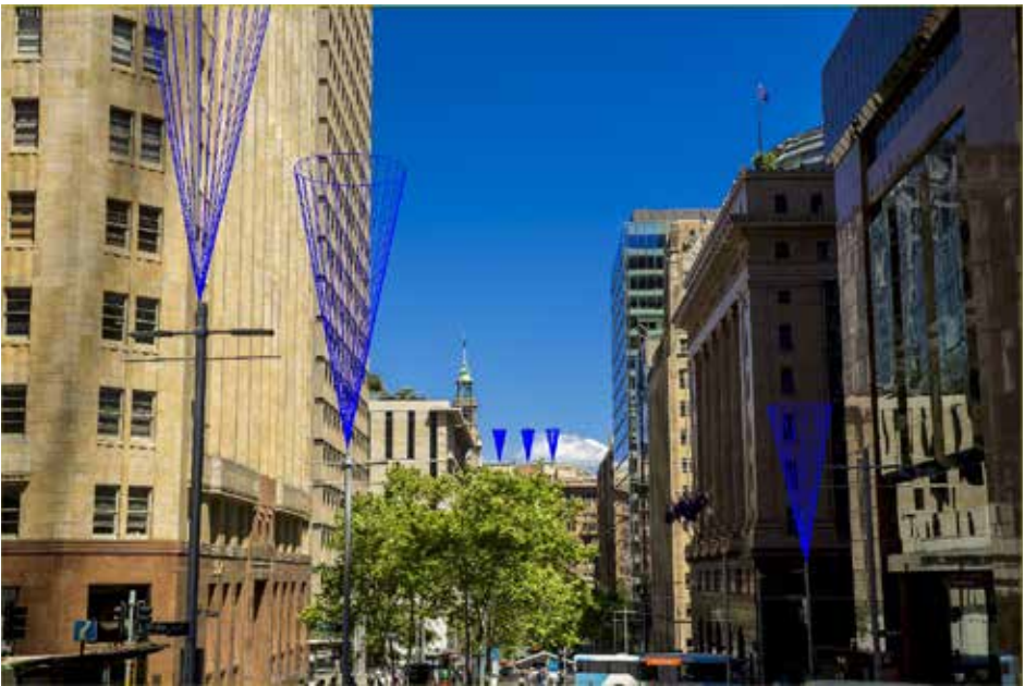
Step 2 - Camera located in 3d model at surveyed location with matched camera attributes (film/sensor format and focal length) and rotated to match other surveyed points within the view.
