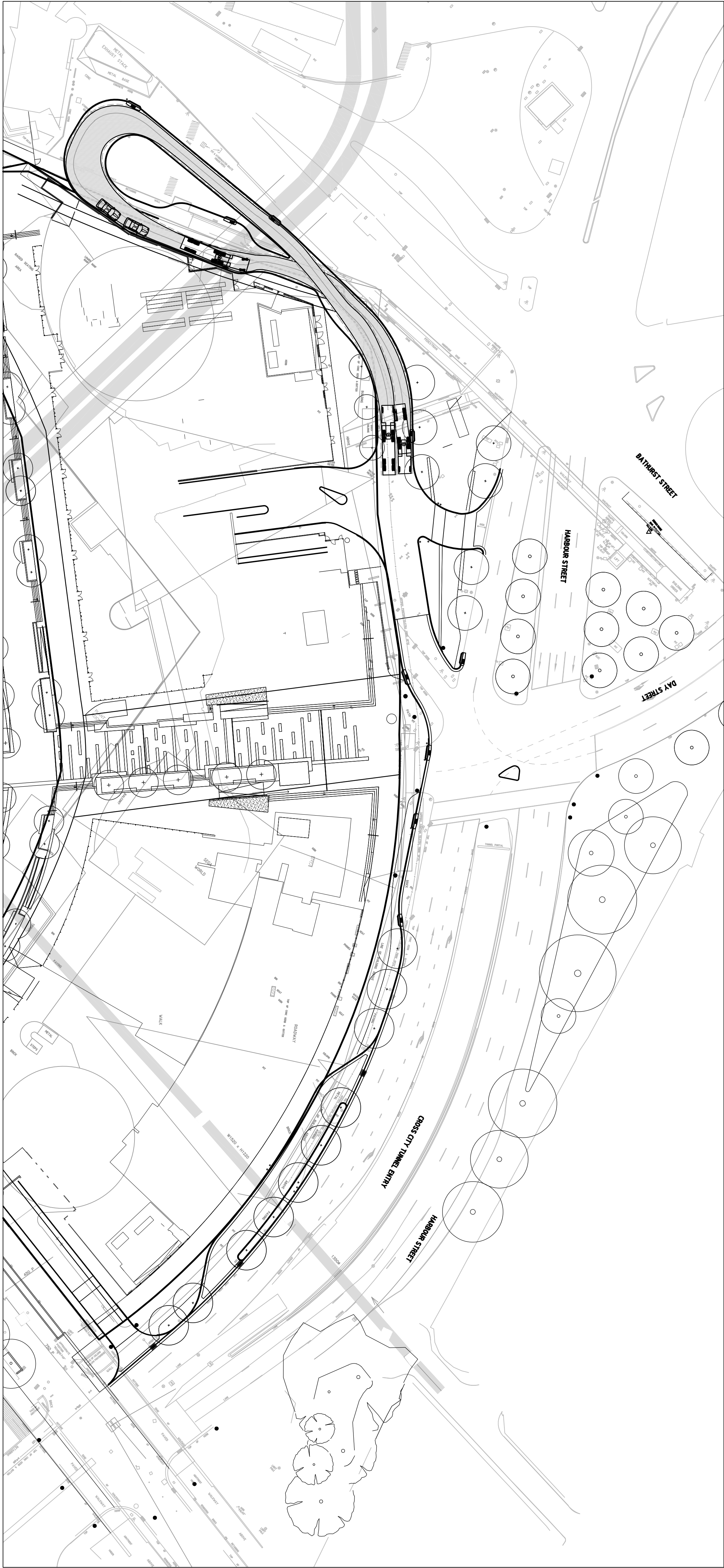
USER DEFINED 14m SEMI TRAILER @ 15Km/h BASED ON AUSTROADS 19.0m SEMI TRAILER VEHICLE TEMPLATE (TRAILER LENGTH REDUCED)
