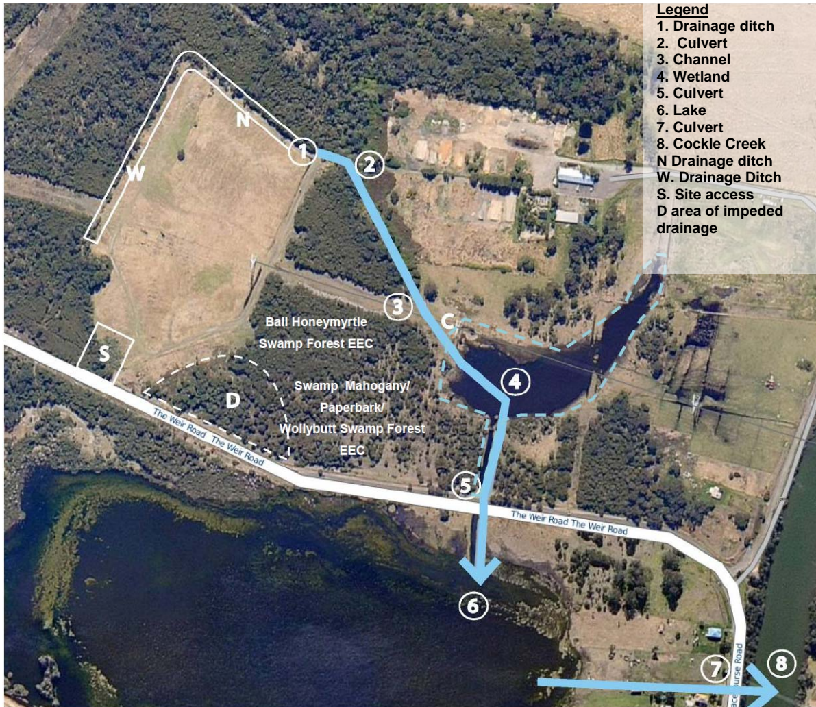
Figure 5: Stormwater flow path
