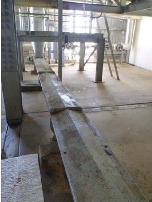
Figure 21 Covered internal conveyor and air collection system
