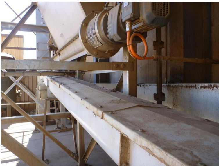
Figure 15 Covered meal cake conveyor prior to storage building
